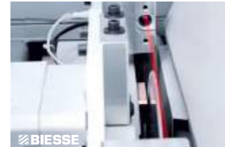
Automatic scoring saw blade alignment system of Selco panel sizing centres.
